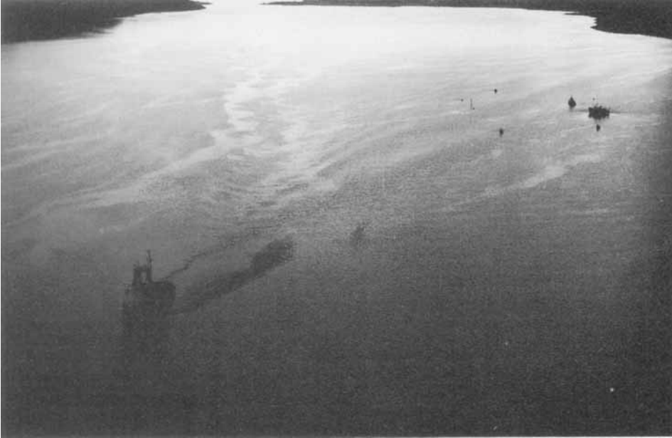
FIGURE 1. The surface effect of an internal wave wake generated by RMAS Roysterer in Loch Linnhe.
